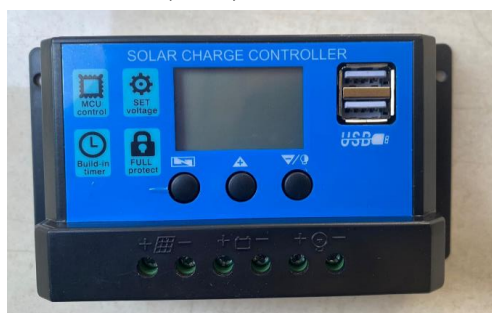
Gambar II. 4 Solar Charge Controller
