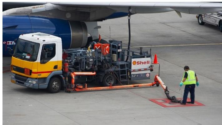
Gambar II. 4 *Refueling and Defueling Truck (RDT)*
