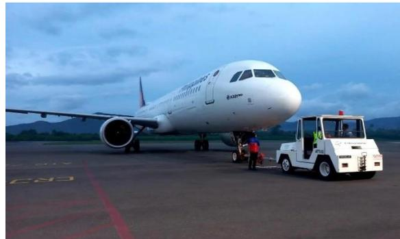
Gambar II. 1 *Aircraft Towing Tractor (ATT)*
