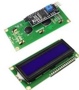
Gambar II. 6 *Liquid Crystal Display (LCD)*
