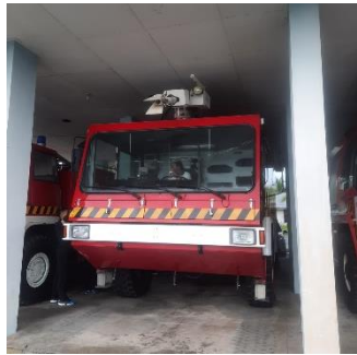
Foam tender type IV Rosenbauer
