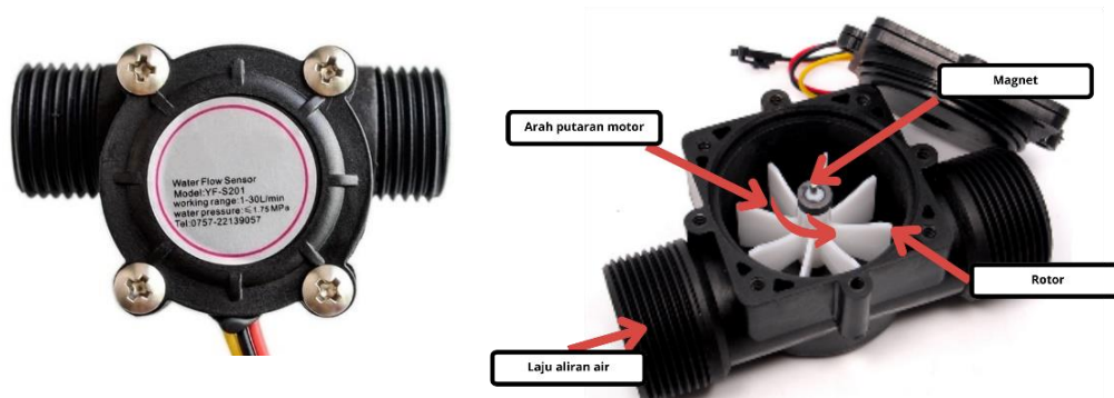
Gambar II. 3 Bagian Water flowmeter
