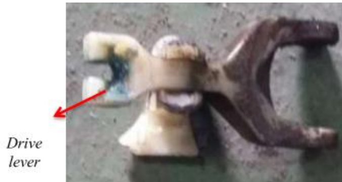
Gambar II. 9 Driver Lever (Tuas Penggerak) (Sumber: Setiawan, 2015)
