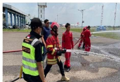
Pengujian Hose Reel Operation
