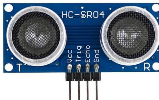
Gambar II. 11 Sensor ultrasonic HC-SR04
