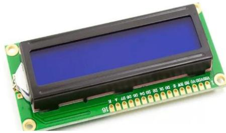
**Gambar II.13** *Liquid Crystal Display*
