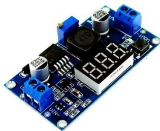
Gambar II. 15 DC Step Down
